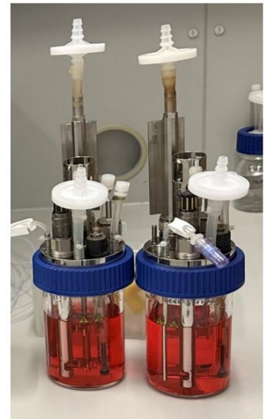
Experimental setup of the DASbox® Mini Bioreactor System (Eppendorf, Germany). Photo: © Kristina Žukauskaitė
